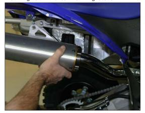
5. Tighten the 4 6x14mm V.A.L.E. Cap screws.
