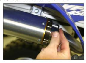
6. Before you run the atv, clean off all fingerprints and dirt, as any oily residue will etch the metal and become somewhat permanent when the system gets hot. Run the atv and enjoy. It is normal for some white smoke to appear the first time you start the bike. This is packing/manufacturing oil from inside the pipe burning off. After 30-60 minutes of use, recheck all fasteners for tightness.
