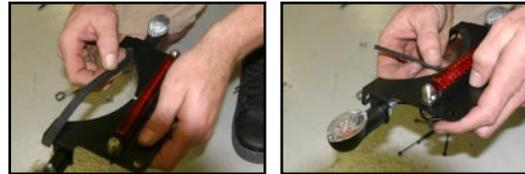
5. Attach the bracket to bottom of Two Brothers exhaust clamps.
