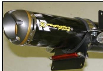
6. Run wires up from fender along left side and use zip ties and zip tie tabs to secure away from muffler.
