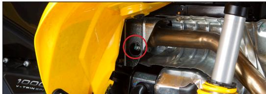
2. Loosen joint bolt and remove rear bumper.
