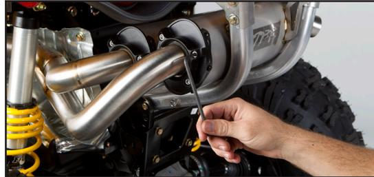
11. Tighten barreled clamp at joint.
