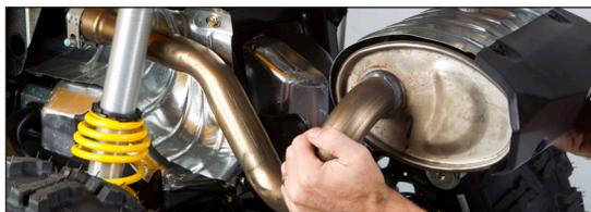
5. Loosely attach TBR muffler to TBR slip tube.
