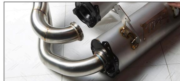
6. Loosely install barrel clamp to slip tube end.
