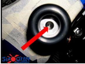
7. We put a bolt through the puck and lightly threaded into the bike. A pencil was then used to draw our diameter of desired shaped hole. A flexible hole template can also be used for the same purpose. Place the hole template on center of the pilot hole (or spot tool) and draw your desired diameter.
