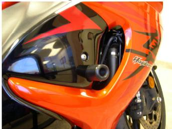
10. Remove left side bolt. Mount left side puck with (99-HB-SH10125090) Socket Cap 10 X 1.25 X 90 Main Engine Stud and torque down.
