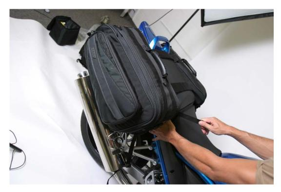
**Step 15:** Route the strap through a secure mounting point on the chassis and back to the female clip.
