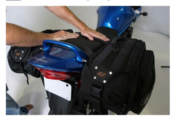
**<u>Step 3</u>**: Use adjustable strap from one bag to secure to the other. Never route the strap under the wheel fender.
